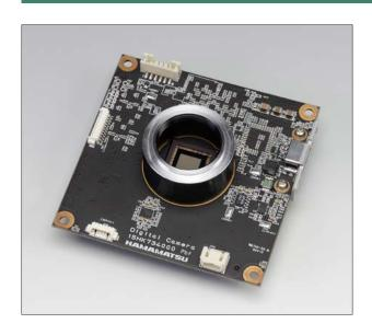
The core of the C13770-50U camera is the scientific image sensor, an advanced CMOS detector that simultaneously achieves high resolution, fast readout speeds and low noise. With its small size, board-level design and simple, low-cost integration using USB 3.0, the C13770-50U is the ideal camera for OEM scientific imaging.
